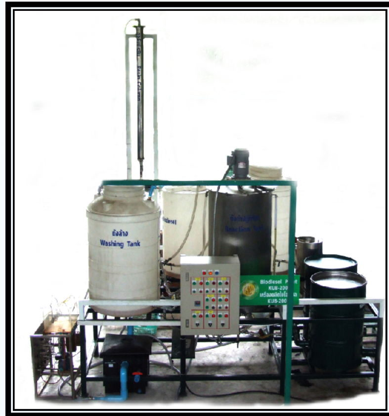
150 L of biodiesel reactor from Kasetsart University
