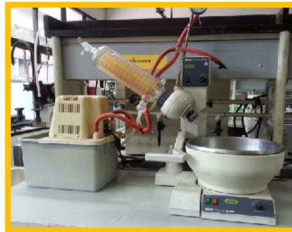
Evaporation to °Brix of sugar
